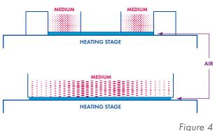
Air gaps and temperature control Air is a poor energy conductor, and gaps between the medium and heated surface will cause temperature variation.
