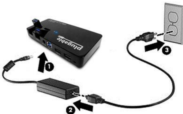
Pictured: Connections For USB Hub to Power Source
