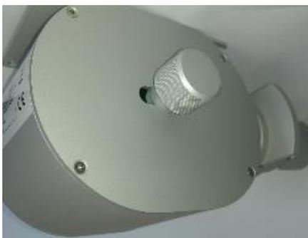
The knob for adjusting the mirror is placed on the left hand side of the Light Source. The rotatable mirror has two different sides. One side is a plane mirror, while the other is concave.
