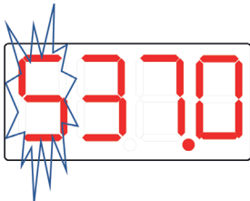
Figure 6 Flashing Display in Set Point Mode
