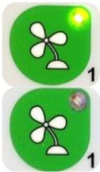
Press the “1- Fan Velocity” button to turn the fans ON. When activated a small green light on top of the button will switch on.
