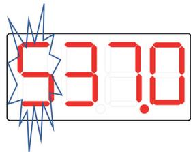
**Figure 6** Flashing Display in Setpoint Mode
