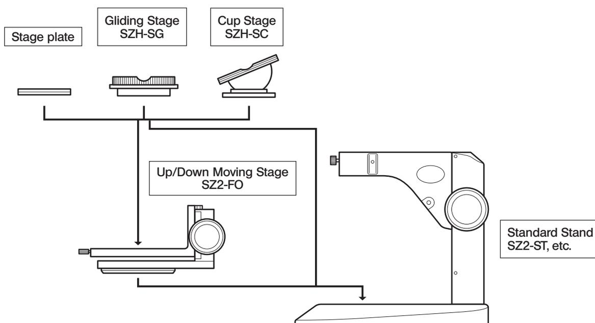
◎ When using a filter or simplified polarized light system in combination with the transmitted illumination stand, mount the filter holder or polarizer on the stand before installing the up/down moving stage.
