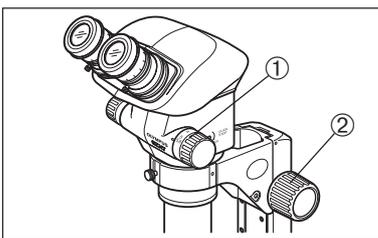
©When the optional AS unit (SZX-AS) is used, the contrast of image and the focal depth of specimen can be adjusted with the aperture iris diaphragm lever.
