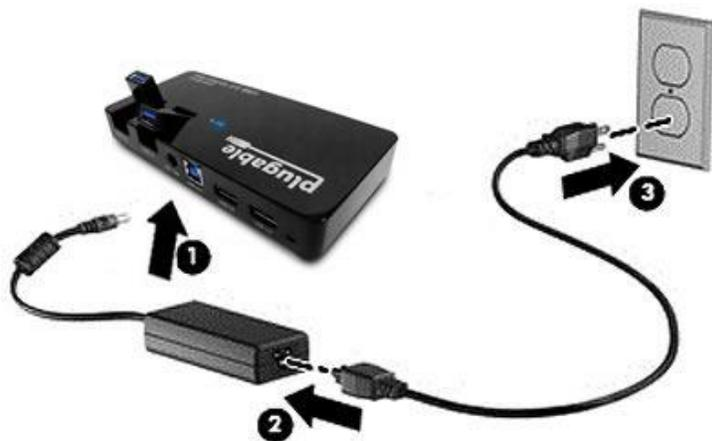
**Pictured: Connections For USB Hub to Power Source**
