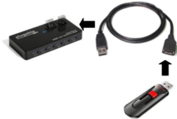
**Pictured: USB Drive Connected to Hub**
