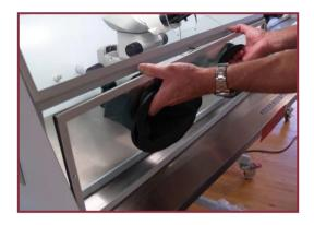
Panel removed and clear access for cleaning.
