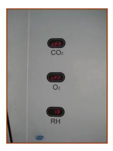
When Fan is switched ON the actual gas concentration for  $CO_2$  and  $O_2$  will be displayed only if  $CO_2$  and  $O_2$  regulators have been activated in the menu.
