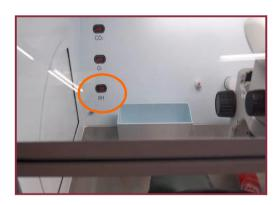
If the alarm sounds either move the reservoir to the non-warmed area or remove the reservoir from the working area. If the G603 is not in use vent the working area by opening the side hatches.
