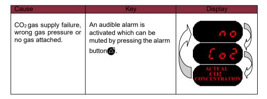
**Note:** The message will be shown in the upper display placed in the inner wall
