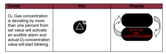
**Note:** When there is an alarm an acoustic signal is also activated which can be muted by pressing the alarm  $\triangle$  button.
