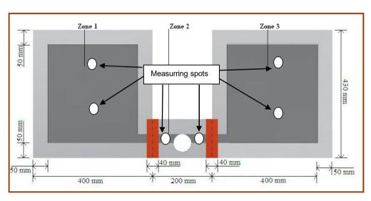
There are three different temperature sensors that may need to be calibrated. Each zone most be calibrated separately. To calibrate "zone-1", measure only temperature in "zone-1".
