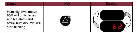
**Note:** The humidity alarm will also go on even if the unit is switched OFF. This
