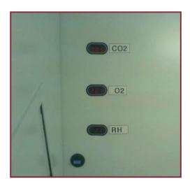
The first display from the top is used to show the status of the CO<sub>2</sub> regulator (ON or OFF) and to show the actual concentration of CO<sub>2</sub>. This display is also used to alert the user in case of any alarm that is related to the CO<sub>2</sub> regulator, wrong CO<sub>2</sub> concentration or wrong incoming gas pressure).
