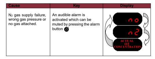
**Note:** The message will be shown in the middle display placed in the inner wall
