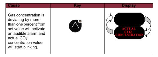
**Note:** When there is an alarm an acoustic signal is also activated which can be muted by pressing the alarm button.
