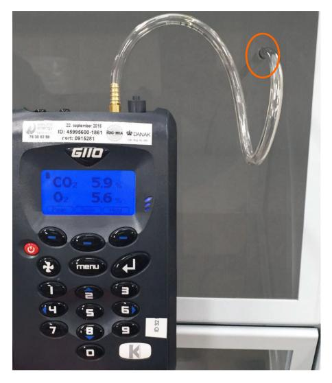
Compare the CO<sub>2</sub> readout with the value shown under 'CO<sub>2</sub>' in the menu and adjust if necessary.
