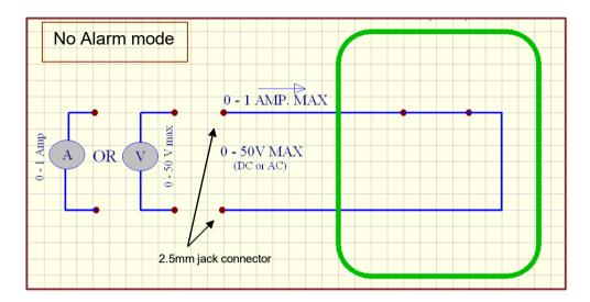
Whenever the G603 goes into an alarm mode the switch will become 'open circuit'.
